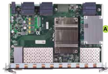
A x86 control board
