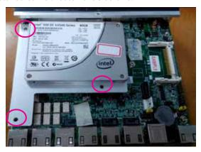
6. Connect SATA cable between the SSD and the motherboard.
