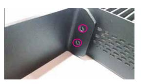
4. Attach the ears of the L-shaped brackets to the rack and then apply long threaded nails.
