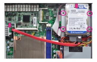
**Note**: Please note the original package only includes one SATA cable (data), You need to order another cable (SATA data cable or data+power cable) for additional SATA HDD installation.
