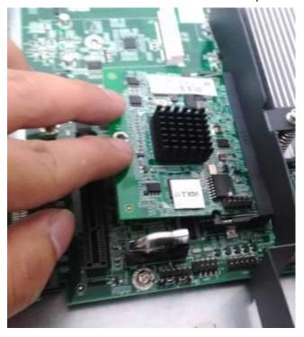
3. Apply a screw to secure the IPMI card.
