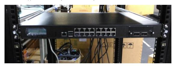
4. To slide the appliance out, gently pull it outwards. Then, press the slide-rail locks on both side and slide the appliance out.
