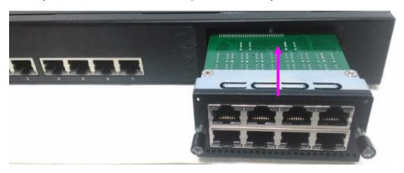
4. Secure the module with two captive screws on the bezel.
