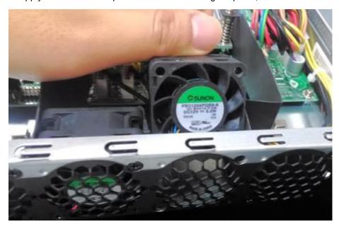
3. To install a new one, just place the new fan to the original place and apply two screws.
