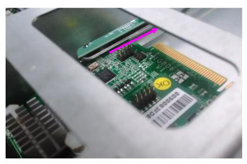
3. Slide your Ethernet NIC module into the space, until it is firmly attached.
