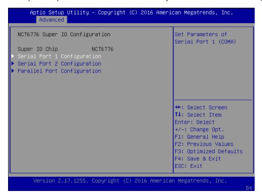
Press "Enter" to enable or disable the Serial Port 1 (COMA). Device setting is fixed as default.
