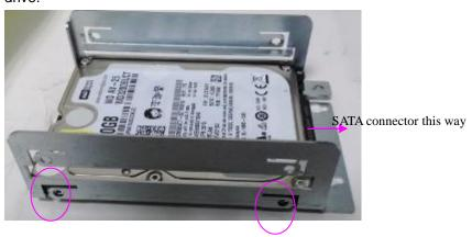
5. Place the tray with HDD/SSD installed back to its original spot inside the system. Remember to aim the two latching holes. Then slide the tray upwards to get it locked by the two latching spots.
