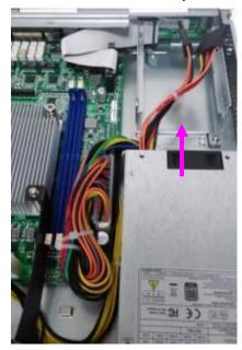
2. Slide the tray downwards. Then the tray will be loosened from the two latching spots.
