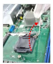
Locking Plate **3.** When you extract the processor from its package, carefully hold it by its edges and avoid touching its golden contacts side. Make sure the golden triangular mark is aligned with the white one marked on the motherboard and then insert it into the socket, as indicated in the picture.
