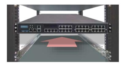
To detach the chassis from the rack, pull the Release Tabs on both sides of the brackets towards you while gently sliding the chassis out.
