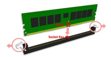
**4.** Push the module down into the slot until it is firmly seated. Press vertically on both corners of the card until it clicks into place.
