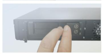
**7.** Lock the tray with the provided key. Turn the key 90° clockwise to the "Locked" position.
