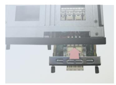
**4.** Once the module is firmly seated, rotate clockwise and tighten the two lock-screws.
