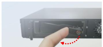
Push the SSD into the slot, with its SATA contact facing inward.
