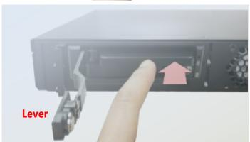
Push the lever back to close the slot; the mechanism of the caddy will have the SDD connected into the socket automatically.
