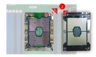
**3.** Flip the PHM over, with the package land of the processor facing the socket, carefully hold the PHM while lowering it vertically to engage it to the alignment pins of the bolster plate.
