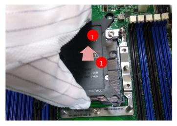
**2.** Flip the PHM over to align PIN1 of the carrier with the Cutout of the bolster plate.
