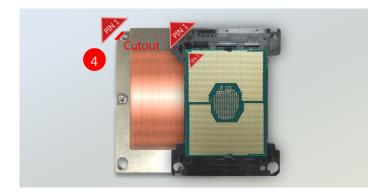
**5.** With a little pressure, push the four corners of the carrier down to engage their latching features with the corresponding corners of the heat sink. You might hear a clicking sound when the latch clicks into place.
