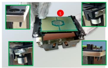
**6.** Go through the four corners to check if the latches are engaged. If correctly latched, the corners of the carrier should be tightly attached to the heat sink, and no gap in-between is observed.
