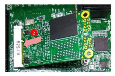
**3.** Push down on the module and secure it with screws that come with it.
