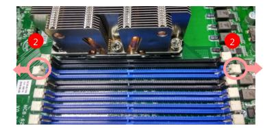
**3.** Align the notch of the DIMM module with the socket key in the slot.
