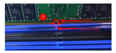
**4.** Insert the module into the slot until it is firmly seated. The motherboard of NCA-6210 is designed with <u>20</u> DDR DIMM sockets.
