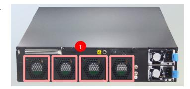
**2.** Loosen the two lock-screws of the fan you would like to replace.
