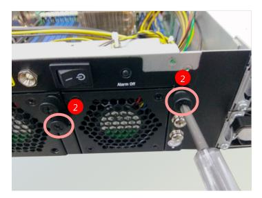
**3.** Hold onto the two lock-screws and pull it out.
