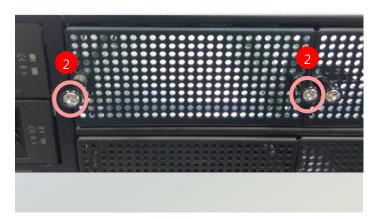
**3.** Remove the door and locate the PCIe socket for module insertion.
