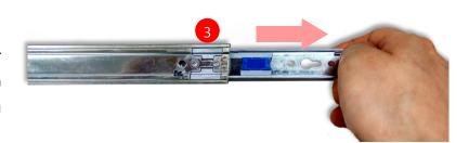
**5.** Align the bracket to the side of the chassis and make sure the screw-holes are matched, and then secure the bracket onto the chassis with five provided M4X4L screws.
