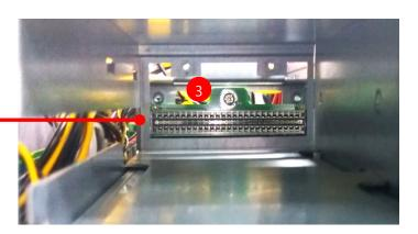
**4.** Insert a new power supply unit. Push the unit in until it clicks into place.
