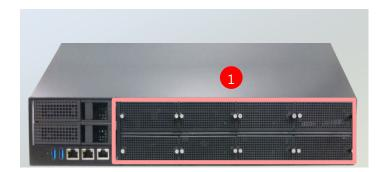
**2.** Rotate clockwise and loosen the two lock-screws.
