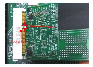
**2.** Insert the module at 30 degrees into the socket until it is fully seated in the connector.
