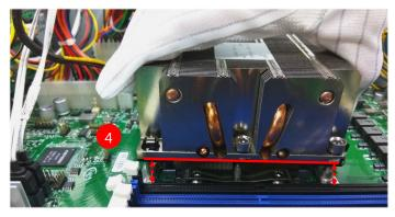
5. Use a torque driver to tighten the four nuts to 12 in-lbf into the bolster plate following the sequence indicated on the heat sink (#1→ #2→#3→#4).
