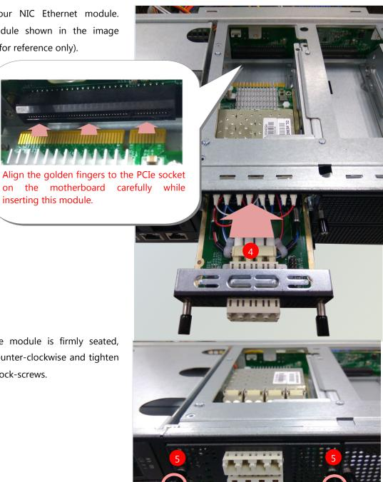
5. Once the module is firmly seated, rotate counter-clockwise and tighten the two lock-screws.
