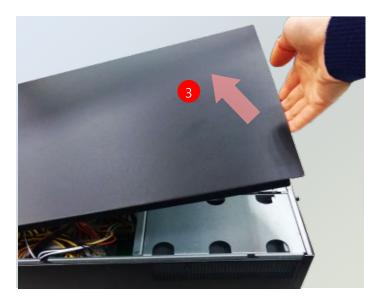
**4.** Remove the cover that protects the CPUs and the fans.
