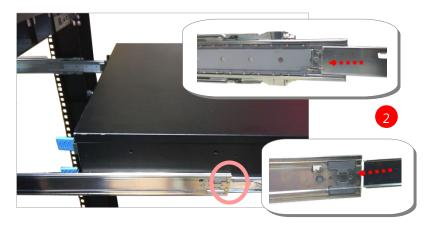
While pushing in the system, please also push and hold the Rail Lock tab on both brackets.
