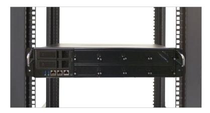
13. To remove the system from the rack, gently pull it outwards towards you while pushing the Release Tab on both sides of the brackets.
